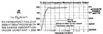
Note that some 2 to 3 dB of maximum output in the 30 to 45 Hz range is sacrificed when the step-down mode is used.
