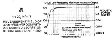
Note that some 2 dB of maximum output in the 40 to 70 Hz range is sacrificed when the step-down mode is used.
