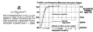
Note that some 2 to 3 dB of maximum output in the 60 to 90 Hz range is sacrificed when the step-down mode is used.
